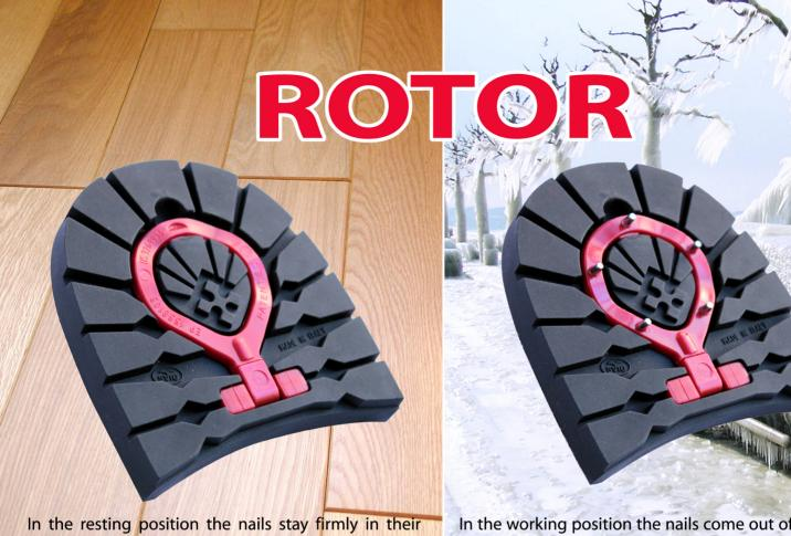
In the resting position the nails stay firmly in their slots, sunk in rubber. Rubber is the only element that touches the floor. Nails can be easily removed from resting position with your bare hands; if the sole is dirty you can simply use a pen, a key, or a hook which can be supplied separately.
